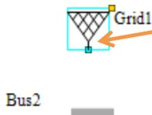
Click and drag the symbol to make the connector handle touch the bus. Just before the touch, press the “Ctrl” key and they will connect.
