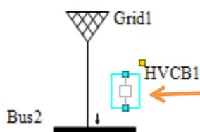
For protective devices, simply move the device to touch the connector line while holding down the ‘Ctrl’ key.
