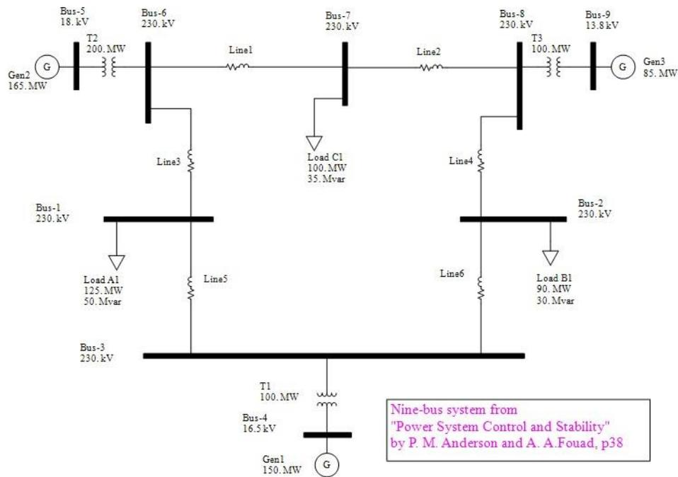
After running a power flow calculation, the results will also be displayed on the drawing, as shown below. As you can see, the results below match the above calculations from the book.
