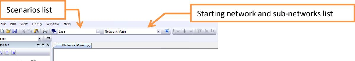
The “Base” list is the scenarios list. Each scenario can have different device statuses (on/off, or in-service/out-of-service), and page-wide datablock or protective device statuses (hide/show). The “Network Main” list contains all pages, including the starting network and all sub-networks
