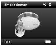
Fig. 4 Smoke Sensor icon in Home Center 2 indicating the smoke alarm and a tamper alarm*
